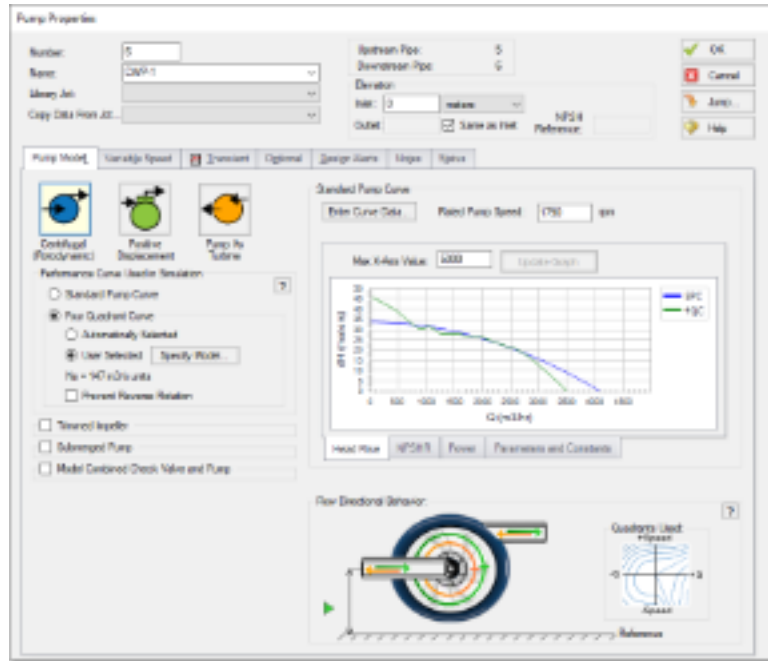
Figure 4.5 Pump Model tab defined using the Four Quadrant Curve, where the Flow Directional Behavior section shows the pump behavior for different flow and speed cases
