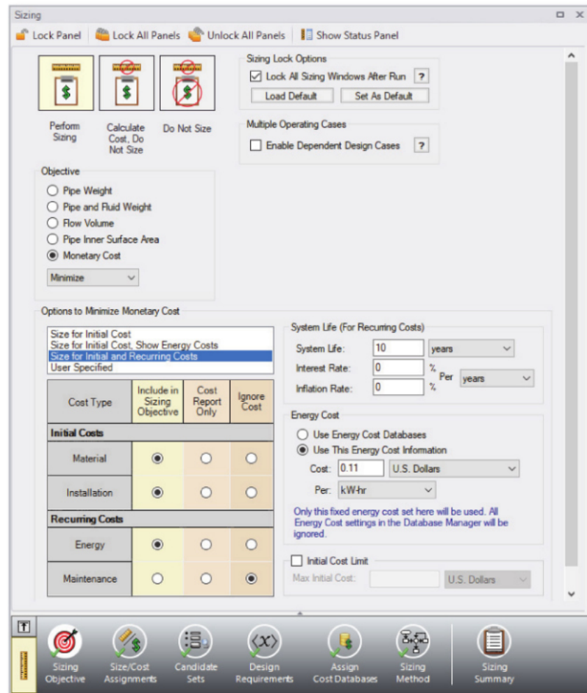
Figure 3.23 Sizing Objective defined for life cycle cost sizing – Energy cost in table was moved from the “Cost Report Only” column to the left column “Include in Sizing Objective”
