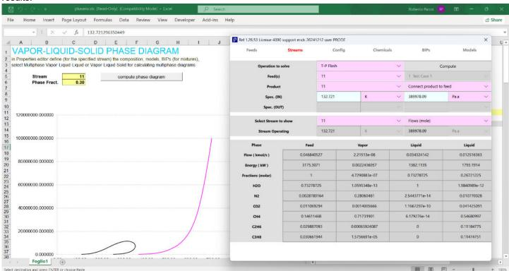
for this mixture including a large fraction of Water the graph shows vapor-liquid-liquid (black) and vapor-liquid (red) lines.
