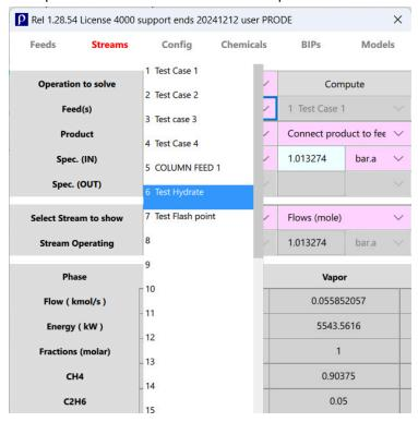
Prode Editor allows to solve flash operations with different specifications, as example we model a control valve wih Pin 30 Bar.a, Tin 280 K and Pout (10 Bar.a) , the valve is modeled as adiabatic stage (dH = 0.0) and the solver will calculate Tout, n Prode Editor, Streams tab :
