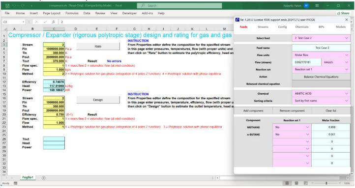
this page allows to design and rate polytropic stages (centrifugal compressors) also including phase equilibria (two phases operations), the procedure allows to select different methods.
