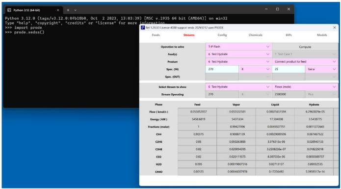
The library allows to solve unit operations as centrifugal compressors (rigorous solution of polytropic stages including phase equilibria), safety valves (with HEM, HNE, HNE-DS... models), pipes etc.
