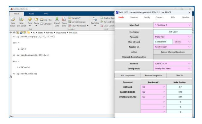
In the same way you can solve a polytropic stage (centrifugal compressor) giving the initial conditions (t=330K, p=200000 Pa) , final pressure (4000000 Pa), model (1) and efficiency (0.75), see the description of method PSPF() for additional information and details about the models available
