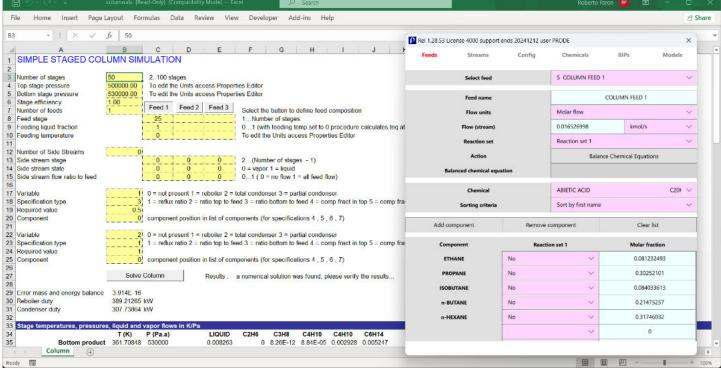
The page allow to define the type of column, the operating conditions, the feeds and the specifications, click on Solve Column button to solve the column and show operating conditions and compositions on the different trays.
