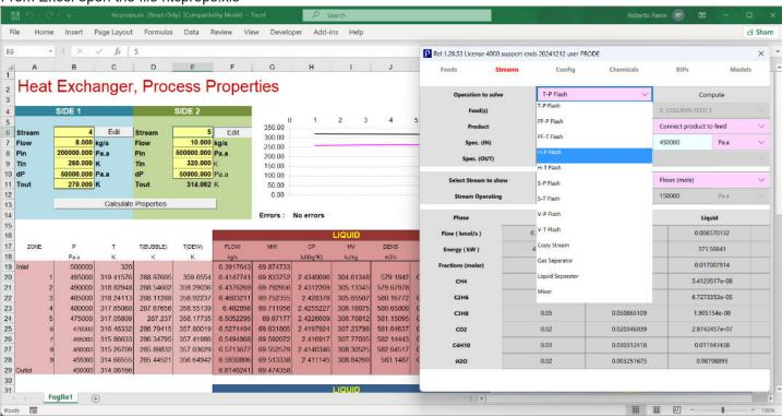
on the different sides there are the buttons Edit to access Prode Editor and define / edit the compositions, the models, the units of measurement, settings etc. in addition, Prode Editor allows to solve directly many different flash operations.
